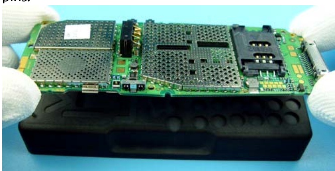
Lift the Engine Module with the new Domesheet from the Jig.
