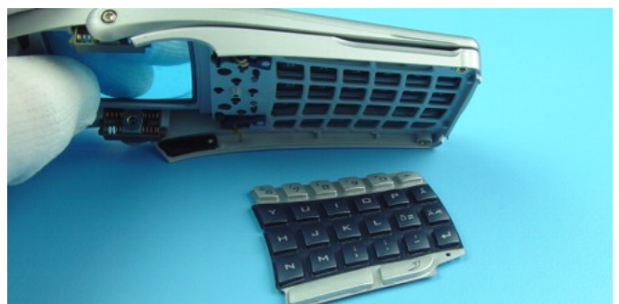
Keymat drops out when turning A-Cover.
