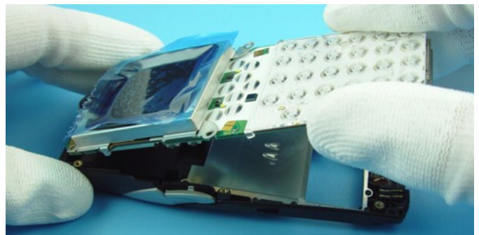
Lift the engine from B-Cover.
