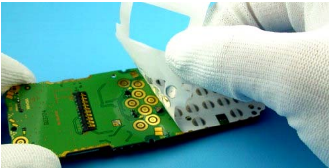
Remove the defective Domesheet carefully.
