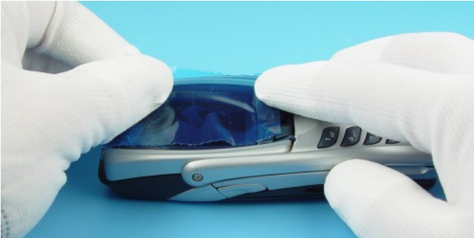
Protect LCD window to avoid dust and scratches.
