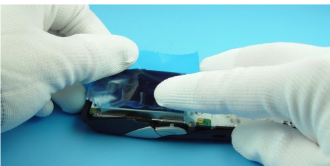
Protect LCD to avoid dust and scratches.
