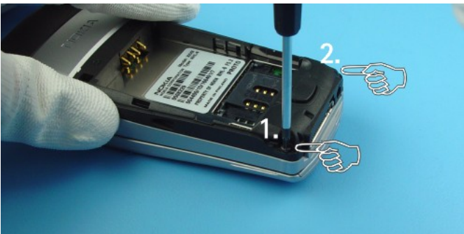
Unscrew the two TORX PLUS® size 6 screws, using the order shown. For assembly, the reverse order and a torque of 17Ncm have to be used. Use always new screws.
