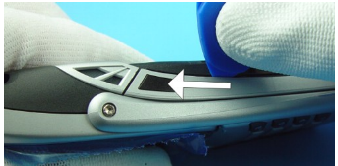
Place the SRT-6 between B-Cover and A-Cover, and shift it carefully as shown in the picture. Note the correct position of the SRT-6, tip should not touch the PWB.
