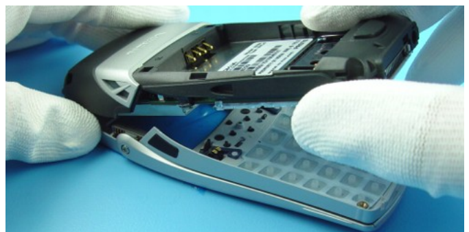
Separate the engine from A-Cover.
