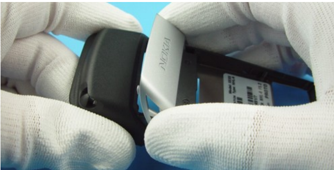
After releasing of the snaps, the Logo Bracket can be removed.
