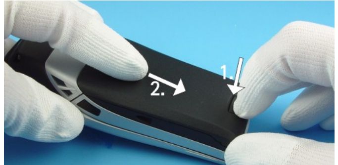
Press Release Button before removing Battery Cover.
